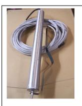
The C400 borehole microseismicity monitoring sensor
